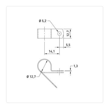
Bundle Diameter [mm]: 12,7 Color: Natural Distance Middle/Middle [mm]: 14.1 UL94-V2 Flammability Class: Material: PA 6.6 Material Group: Plastic Mounting Hole [mm]: 5.2 Thickness [mm]: 1.3 Width [mm]: 12.7 1.17g
