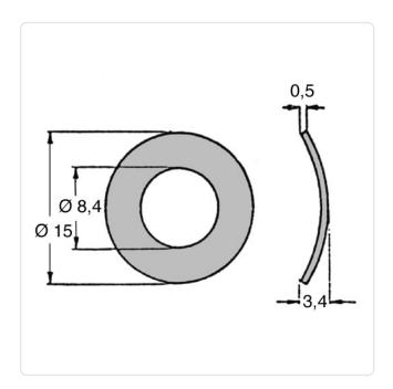
DIN/ISO: DIN137A Finish: Plain For Thread Size: M8 0.5 Height [mm]: Inner Diameter [mm]: 8.4
