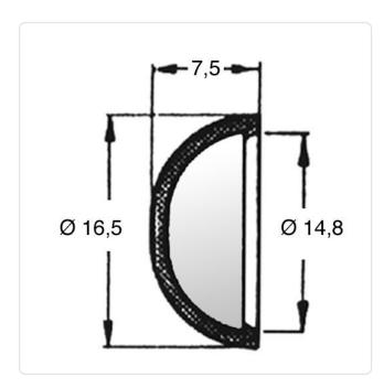
Color: Gray 7.5 Head Height [mm]: Inner Diameter [mm]: 14.8 PA 6.0 Material: Material Group: **Plastic**
