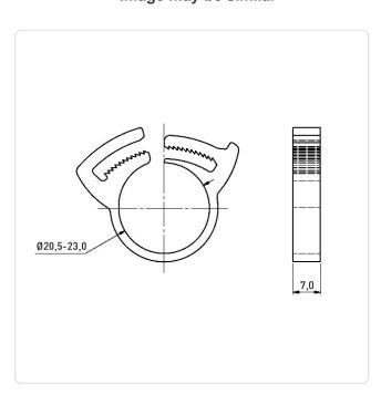
Color: Black Flammability Class: UL94-V2 PA 6.6 Material: Panel Thickness Range [mm]: 20,5-23,0
