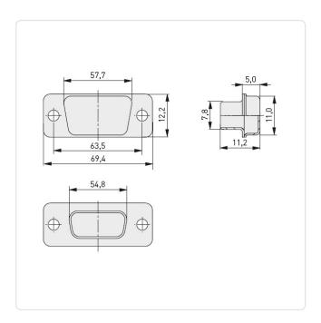
Material: Steel Steel Material Group: Model: D-Sub Mounting Hole [mm]: 3.2 Width [mm]: 69.4 Weight: 7.38g
