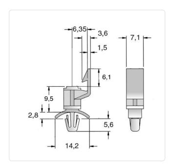
Color: Natural Flammability Class: UL94-V2 Length [mm]: 9.5 Material: PA 6.6 Plastic Material Group: Panel Hole Ø [mm]: 4.8 Panel Thickness [mm]: 0,8-2,0
