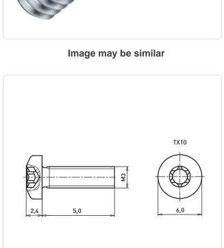
Actuator Size: Torx T10 DIN/ISO: ISO14583 Drive Type: **TORX**
