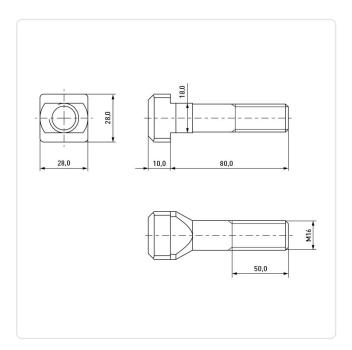
DIN/ISO: **DIN787** Plain Finish: Head Height [mm]:
