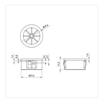
Color: Black Inner Diameter [mm]: 20.6 Material: PA 6.6 Material Group: Plastic Max. Panel Thickness [mm]: 3.2
