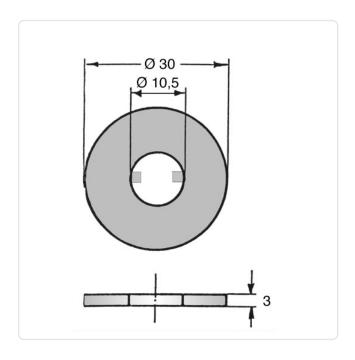
Color: Natural For Thread Size: M10 Height [mm]: Inner Diameter [mm]: 10.5 Material: PA 6.0 Material Group: Plastic Outer Diameter [mm]: 30 Weight: 1.95g
