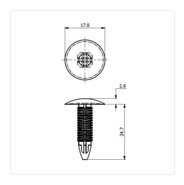
Color: Black Flammability Class: UL94-V0 Head Diameter [mm]: 17.8 Head Height [mm]: 2.6 Length [mm]: 24.7 Material: PA 6.6 Material Group: **Plastic** Mounting Hole [mm]:
