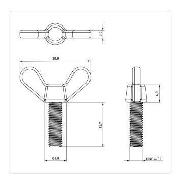
Color: Natural Flammability Class: UL94-V2 Head Diameter [mm]: 20 Length [mm]: 12.7 Material: PA 6.6
