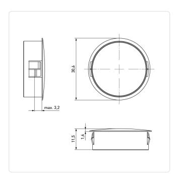
Color: Black Flammability Class: UL94-V2 Head Diameter [mm]: 30.6 Head Height [mm]: 1.6 PA 6.6 Material: Material Group: Plastic Snap-In Model: Mounting Hole [mm]: 25.4
