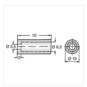
Color: Black Flammability Class: UL94-HB For Thread Size: M3.5 Inner Diameter [mm]: 6.2 Length [mm]: 10
