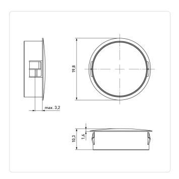
Color: Black Flammability Class: UL94-V2 Head Diameter [mm]: 19.8 Head Height [mm]: 1.6 PA 6.6 Material: Material Group: Plastic Snap-In Model: Mounting Hole [mm]: 17.5
