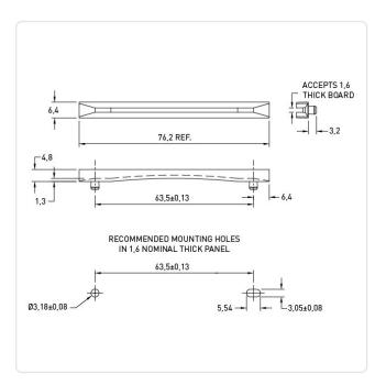
Color: Natural Dist. Mounting Holes [mm]: 63.5 Flammability Class: UL94-V2 Length [mm]: 76.2 Material: PA 6.6 Material Group: **Plastic** Model: Plug-In Foot
