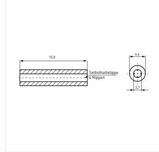
Color: Gray Flammability Class: UL94-V0 For Thread Size: M3 Inner Diameter [mm]: 3.7 Length [mm]: 15 Material: PVC - Polyvinyl Chloride Material Group: Kunststoff Outer Diameter [mm]: 6.4 Weight: 0.51g Conformities: Reach RoHS SVHC
