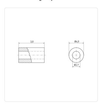
Color: Black Flammability Class: UL94-HB For Thread Size: M2.5 Inner Diameter [mm]: 2.7
