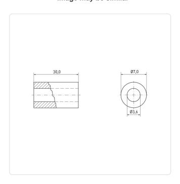
Color: Black Flammability Class: UL94-HB For Thread Size: M3.5 Inner Diameter [mm]: 3.6 Length [mm]: 30
