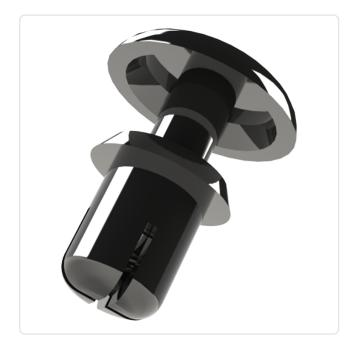
Color: Black UL94-V2 Flammability Class: Head Diameter [mm]: 7.8 Head Height [mm]: 1.9 Length [mm]: 6.1 Material: PA 6.6 Material Group: Plastic Model: removable Mounting Hole Range [mm]: Ø 4.1-4.2 Panel Thickness [mm]: 3,5-4,5
