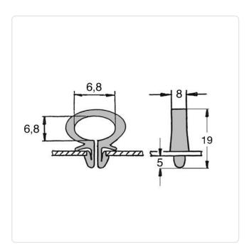
Bundle Diameter [mm]: 5,0-10,0 Color: Black Height [mm]: 17 Material: PA 6.6 Material Group: **Plastic** Mounting Hole [mm]: 6.5 Panel Thickness [mm]: 2,5-4,0 Width [mm]: Weight: 0.57g
