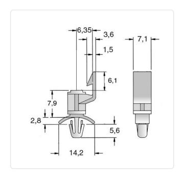
Color: Natural Flammability Class: UL94-V2 Length [mm]: 7.9 Material: PA 6.6 Material Group: **Plastic** Panel Hole Ø [mm]: 4.8 Panel Thickness [mm]: 0,8-2,0
