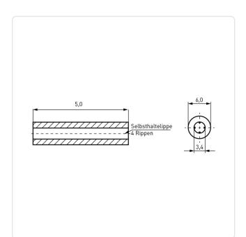
Color: Black Flammability Class: UL94-V2 For Thread Size: М3 Inner Diameter [mm]: 3.4
