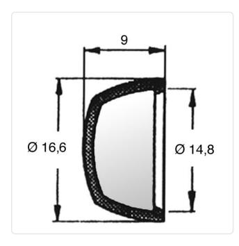
Color: Gray Head Height [mm]: 9 Inner Diameter [mm]: 14.8 Material: PA 6.0 Material Group: **Plastic**
