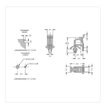
Color: Natural Flammability Class: UL94-V2 12.2 Length [mm]: PA 6.6 Material: Material Group: **Plastic** PCB Thickness [mm]: 1,6 Panel Hole Ø [mm]: 4.8 Panel Thickness [mm]: 1,0-2,3 Weight: 0.81g
