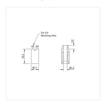
Color: Natural Flammability Class: UL94-V2 For Thread Size: M4 Inner Diameter [mm]: 4.2 Length [mm]: 22.2 Material: PA 6.6 Material Group: Plastic Mounting Hole [mm]: 5.9 Outer Diameter [mm]: 7.1
