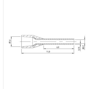
Color: Gray Finish: **Tin-Plated** Insulation: Polypropylene Length [mm]: 10.6 **Electrolytic Copper** Material: Material Group: **Electrolytic Copper** Plug-In Length [mm]: 6 Wire Cross Section [mm<sup>2</sup>]: 0.14 Weight: 0.03g Conformities:
