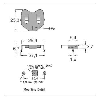
Battery Type: Cell Dia. 24mm
