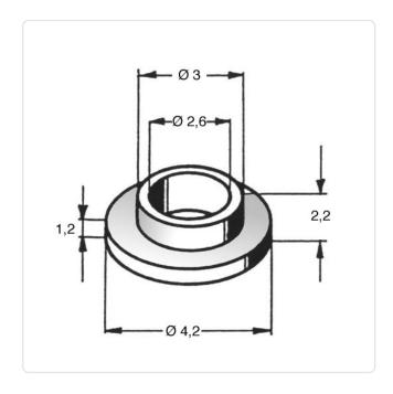
Color: Black Flammability Class: UL94-V0 2.2 Height [mm]: Inner Diameter [mm]: 2.6
