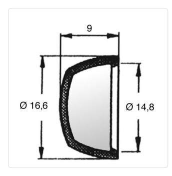
Color: Black Head Height [mm]: 9 Inner Diameter [mm]: 14.8 Material: PA 6.0 Material Group: **Plastic**
