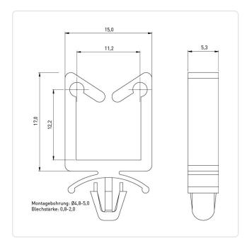
Bundle Diameter [mm]: 10,0-18,0 Color: Natural Height [mm]: 17 Material: PA 6.6 Material Group: **Plastic** Mounting Hole [mm]: 4.8
