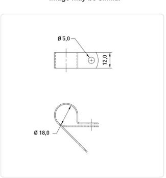
Bundle Diameter [mm]: 18 Color: Black Material: PA 6.6 Plastic Material Group: Mounting Hole [mm]: 5 Width [mm]: 12 Weight: 1.32g
