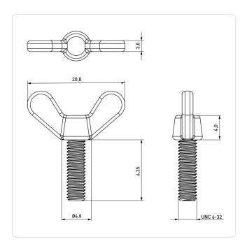
Color: Natural Flammability Class: UL94-V2 Head Diameter [mm]: 20 Length [mm]: 6.35 Material: PA 6.6 Material Group: **Plastic**
