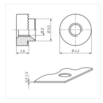
Finish: Plain Height [mm]: 2.8 Material: Steel Material Group: Steel Outer Diameter [mm]: 5.5 Panel Hole Ø [mm]: 4.2 Panel Thickness [mm]: 0,9 - 1,0 Thread Size: М3 Weight: 0.43g
