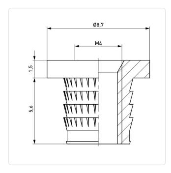
Finish: Plain Head Diameter [mm]: 8.7 Length [mm]: 5.6 Material: Brass Material Group: **Brass** Minimum Edge Distance [mm]: 2.5 Panel Hole Ø [mm]: 5.6 Thread Size: M4 Weight: 1.29g
