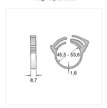
Color: Natural Flammability Class: UL94-V2 PA 6.6 Material: Material Group: Plastic Panel Thickness Range [mm]: 45,5-53,6
