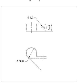
Bundle Diameter [mm]: 50 Color: Black Material: PA 6.6 Plastic Material Group: Mounting Hole [mm]: 5 Width [mm]: 16 Weight: 4.85g
