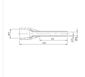
Color: Blue Finish: **Tin-Plated** Insulation: Polypropylene Length [mm]: 13 **Electrolytic Copper** Material: Material Group: **Electrolytic Copper** Plug-In Length [mm]: 8 Wire Cross Section [mm<sup>2</sup>]: 0.25 Weight: 0.05g Conformities:
