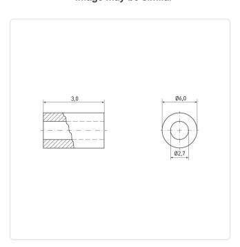
Color: Natural Flammability Class: UL94-HB For Thread Size: M2.5 Inner Diameter [mm]: 2.7 Length [mm]:
