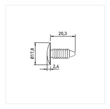
Color: Black Flammability Class: UL94-V2 Head Diameter [mm]: 17.8 Head Height [mm]: 2.4 Length [mm]: 20.3 Material: PA 6.6 Material Group: Plastic Mounting Hole [mm]: 6.4 Panel Thickness [mm]: 3,8-13,6 Weight: 0.6g
