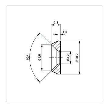
Color: Black For Thread Size: МЗ Height [mm]: Inner Diameter [mm]: 3.2 Material: PA 6.0 Material Group: Plastic Outer Diameter [mm]: 10.5 Weight: 0.17g
