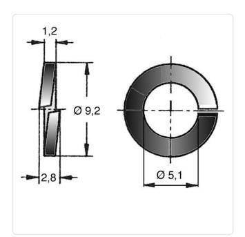
DIN/ISO: DIN127B Finish: Plain For Thread Size: M5 1.2 Height [mm]: Inner Diameter [mm]: 5.1
