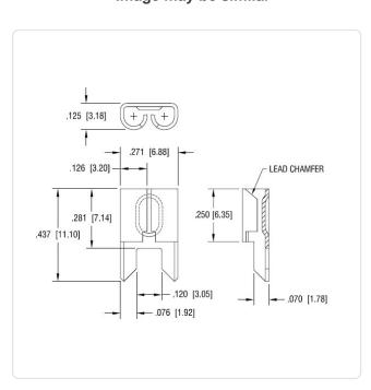
Amperage [A]: 30 5.2x0.64 Fuse Size [mm]: Material: **Brass** Material Group: **Brass** Model: Clip Holder
