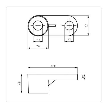
Color: Natural Length [mm]: 6.5 Material: PA 6.6 Material Group: Plastic Panel Hole Ø [mm]: 4.2 Weight: 0.4g
