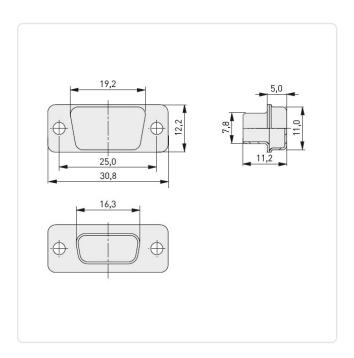
Material: Steel Stahl Material Group: Model: D-Sub Mounting Hole [mm]: 3.2 Width [mm]: 30.8 Weight: 3.1g
