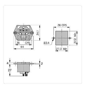
Amperage [A]: 10 Color: Black Connections: 2.8x0.8 Fuse Size [mm]: 5.0x20.0
