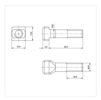
DIN/ISO: **DIN787** Finish: Plain Head Height [mm]:
