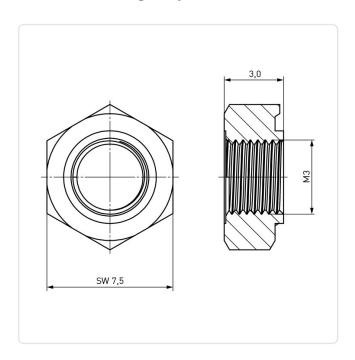
AF / OD [mm]: 7.5 DIN/ISO: **DIN929** Finish: Plain 3 Height [mm]: Material: Steel Material Group: Steel Thread Size: М3 Weight: 0.75g
