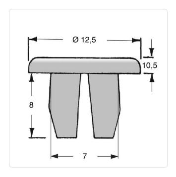
AF / OD [mm]: 12.5 Color: Natural Head Height [mm]: 5 Length [mm]: 8 PA 6.6 Material: Material Group: Plastic Panel Cutout [mm]: 7.0x7.0 Panel Thickness [mm]: 0,5-3,0 Thread Diameter [mm]: Ø 4.2 Weight: 1.14g
