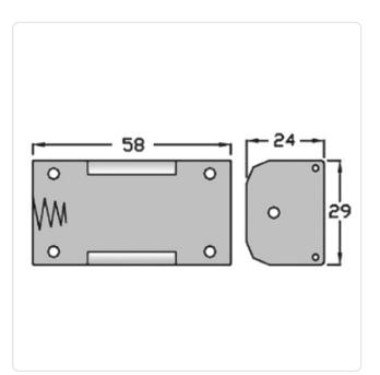
Battery Type: C-Baby Flammability Class: UL94-HB
